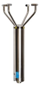
The Gill WindObserver 65 is a precision, solid-state ultrasonic anemometer providing wind speed and direction data via 1 digital and 3 optional analogue outputs and features an IP66 rated stainless steel housing, which is particularly suitable for use in salt-water environments.
