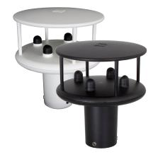
The Gill WindSonic is a low-cost anemometer, which utilises Gill's proven ultrasonic technology to provide wind speed and direction data via one serial or two analogue outputs. To confirm correct operation, outputs are transmitted together with an instrument status code.
